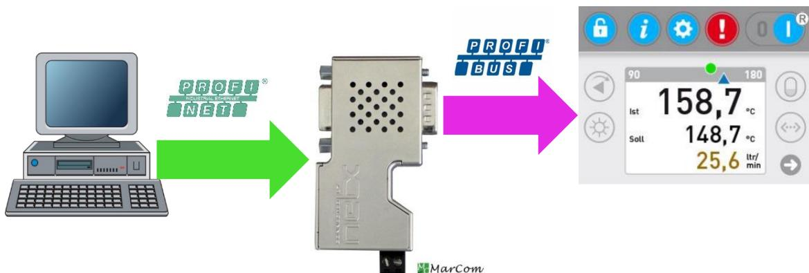
This makes it possible to have the controller monitored and controlled via Profinet by a master (e.g. an industrial or personal computer or SPS).
